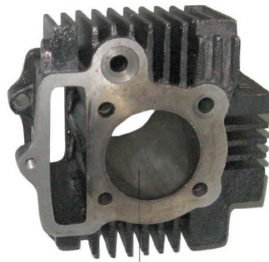
inner cylinder wall
