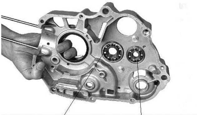
main shaft bearing
