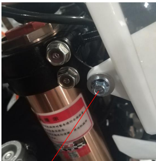
Fixing Bolts on Upper Bracket
