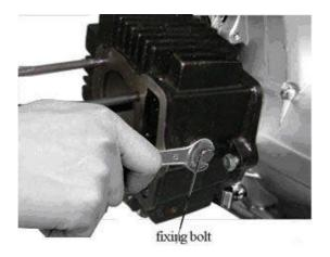
Remove the guide wheel of timing chain to inspect for wear and damage. Replace if necessary.
