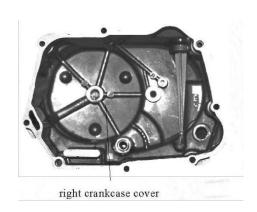
Left view of right crankcase half is shown in figure and check whether bearing of main shaft and countershaft are worn. Replace if necessary.
