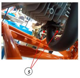
Remove muffler pipe clamp bolt: 3 Remove muffler pipe mounting bolt: 2 Remove muffler pipe 4 Remove exhaust head pipe 1
