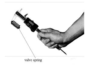
Remove the spring of inlet and exhaust valve to inspect for wear and damage.
