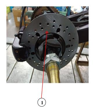
Check the brake pad thickness 2
