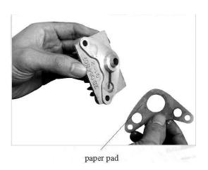
Remove inlet/exhaust valve cap .Check the state of seal ring of valve cap and replace if worn or if reuse is questionable.
