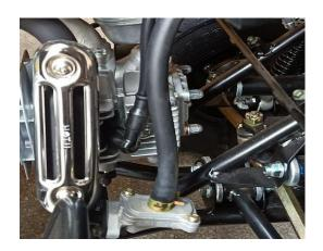
Remove the secondary inlet air cleaner and inspect for wear and damage. Clean and replace if necessary.
