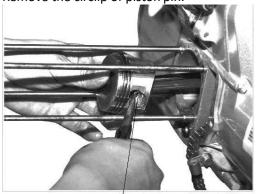
piston pin circlip
