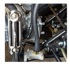
Dismantle the fixing bolt of air pump and check the state of air pump. Replace the air pump if it is worn or if reuse is questionable.
