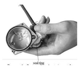
Remove the float needle valve to inspect for wear and damage. Replace if necessary.
