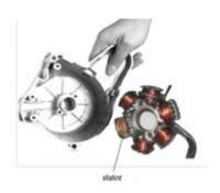
Check stator condition with a multiple-use meter. Replace if damage or can't use.
