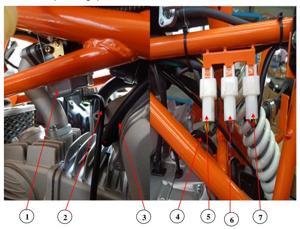
1.Carburetor 2. carburetor overflow hose 3.Starter motor cable 4. Crankcase vent hose 5.Stator/ignition pickup connector 6. Gear indicator connector 7.Voltage regulator connector Note: To inspect the above parts, must remove the shift lever, and left footrest. Please refer to 02-Plastics.
