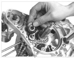
Remove the timing tensioner arm to inspect for wear and damage. Replace if necessary.
