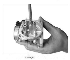
Remove the main nozzle to check whether small hole is clogged. Clean with compressed air if necessary.
