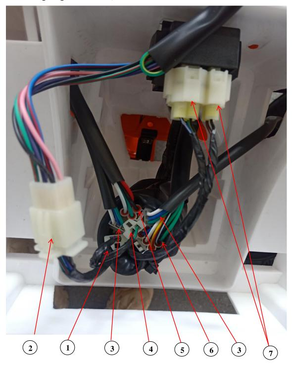
1. Reverse indicator connector(older models 2017 ↓ ) 2. Digital gear indicator connector 3. Headlight connector 4. Neutral indicator connector (older models 2017 ↓ )5. Key switch connector 6. Multifunction switch Connector 7. CDI connector Note: To inspect the above parts, must remove the front rack and hood. Please refer to 02-Plastics.
