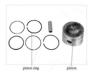
Check the state of piston and replace if worn or if reuse is questionable. Measure diameter of piston skirt. Replace it if the value is beyond the maintenance limit value.
