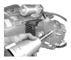
Remove the right cover of cylinder head.
