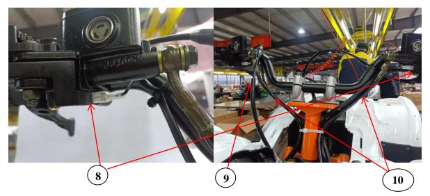
8. Brake switch (left and right) 9. Throttle cable 10. Front and Rear brake lines
