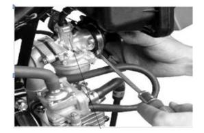
Clean the carburetor as follows: 。 Remove the dirt and clean inner oil way. Dismantle the fixing bolt of float chamber cap.
