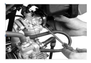
Clean dust on the air filter surface and then dis-assemble the air filter and clean inside.
