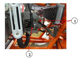
Disconnect gear display connect wire  $(\Rightarrow 1.7)$ Disconnect magneto trigger connect wires  $(\Rightarrow 1.7)$
