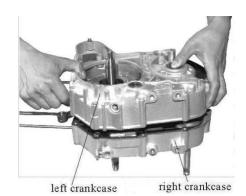
Remove the paper pad to inspect for wear and damage. Replace if necessary.
