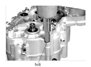
Remove left crankcase half. Take care not to forget the washer of main shaft and countershaft when removing the left crankcase.
