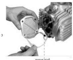
Dismantle the fixing bolt of left cover.
