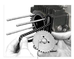
timing driven sprocket
