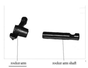
Check the external diameter of rocker arm using a micrometer. Replace the rocker arm shaft if the valve is beyond the maintenance limit valve.
