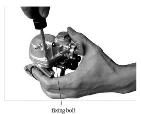
Remove the float chamber cap. Remove the water and debris in the cap if necessary. Check the state of seal ring and replace if it is aging
