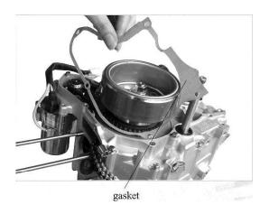
Dis-assemble magneto stator fixing bolt trigger bolt.
