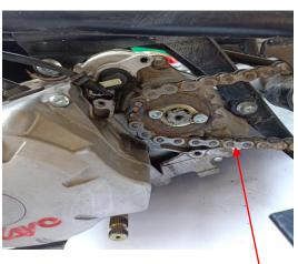
Remove spark plug cap: 2 Disconnect oil cooler hoses banjo bolts: 1, reinsert bolts after lines are removed to prevent oil leaking.
