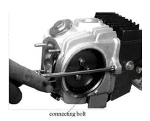
Remove cylinder head assembly.
