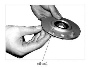
Dis-assemble seal ring and check condition, change if damaged.
