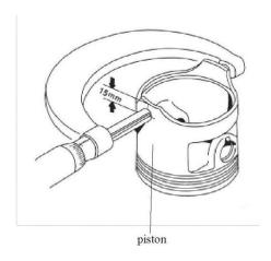
Assemble the piston ring according to the figure and check whether piston ring is damaged or the elasticity is weaken.
