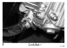
Dismantle suspension bolt of muffler to check whether the suspension support is damaged. Repair or replace if necessary.
