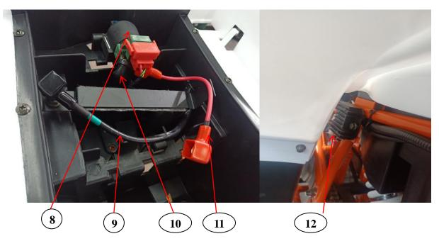
8. Starter Relay 9. Battery negative terminal 10. Starter cable 11. Battery positive terminal 12. Voltage regulator/rectifier
