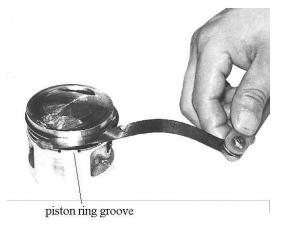
Check whether there is excessive carbon deposit on piston top and groove. Remove if necessary.
