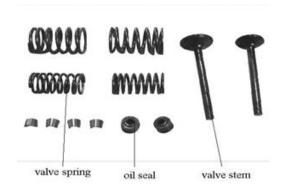
Check the external diameter of valve stem using a wedge. Replace the valve stem if the valve is beyond the maintenance limit valve.
