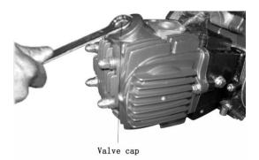
Adjust valve clearance of front cylinder. Turn magnetic rotor counterclockwise to make piston locate at top dead center and make T mark aimed to the mark of left crankcase cover.
