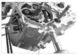
Remove the small timing chain and check the state. Replace if necessary.
