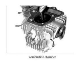
Remove the cylinder head. Pour gasoline into inlet/exhaust pipe to inspect the seal condition. Grind the valve and valve seat if there is gasoline leaking into the combustion chamber.
