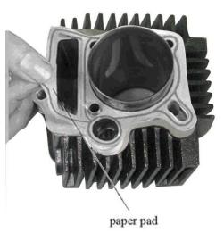
Check whether there is residual gasket on cylinder. Clean with gasoline if necessary.
