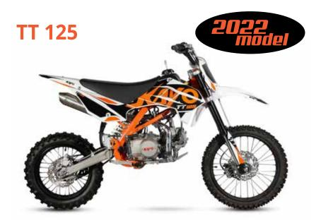
ENGINE **120cc 4-Stroke single** COOLING Air cooled STARTER Electric/Kick FUEL SYSTEM Carbureted TRANSMISSION **4-speed manual** TIRES **70/100-17** front **90/100-14** rear BRAKES Disc brakes, front/rear FRONT SUSPENSION Inverted forks REAR SUSPENSION Single shock
