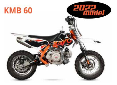
ENGINE **56.8cc 4-Stroke single** COOLING Air cooled STARTER **Electric FUEL SYSTEM Carbureted** TRANSMISSION Fully automatic TIRES **2.50/10** front **2.50/10** rear BRAKES **Disc brakes**, front/rear FRONT SUSPENSION Conventional forks REAR SUSPENSION Single shock
