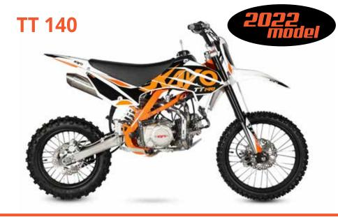
ENGINE 140cc 4-Stroke single COOLING Air/oil cooled STARTER Electric/Kick FUEL SYSTEM Carbureted TRANSMISSION 4-speed manual TIRES **70/100-17** front **90/100-14** rear BRAKES **Disc brakes**, front/rear FRONT SUSPENSION Inverted forks REAR SUSPENSION Single shock
