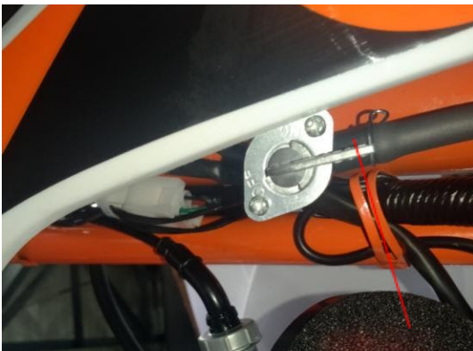
fuel tank switch
