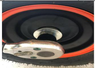
7.Put the front wheel to the steering knot with FBJ all mounting well, use tool ①⑥to lock the nut and washer, then insert the cotter pin(G),, keep the bending angle greater than 180° Note: Torque requirement 77-92N.m
