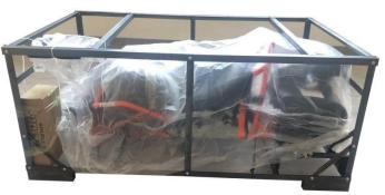
3.Take out the parts attached on the vehicle and the packaging iron frame, remove the iron frame screws, wait for subsequent installation.
