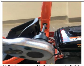
11.Put the rear guard to the fram,use tool ①4to tighten (C). Note: Torque requirement 25-30N.m
