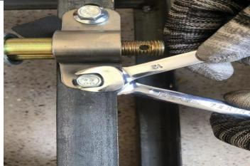
6.Use tool ②③ remove the screws mouning on the rear axle,put the vehicle on the stand for easy installation of other accessories.
