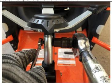
10.Put the steering wheel with the steering column, use tool 153 to lock (D)
