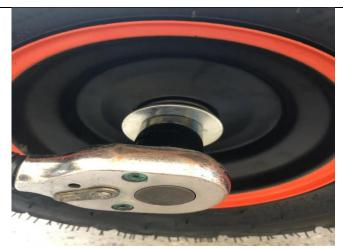
8.Align the rear wheel with the splines(I) and push on the rear axle, with the air nozzle cap facing outward, Use tool ①⑥ to lock the nut (F) and washer (B), then insert the cotter pin (G), keep the bending angle greater than 180° Note: Torque requirement 77-92N.m
