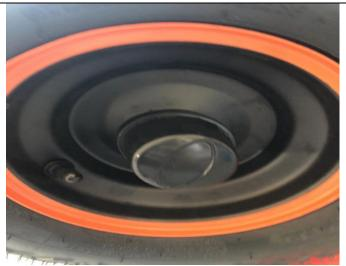
9.Insert the dust cover(A) into the positions shown above.
